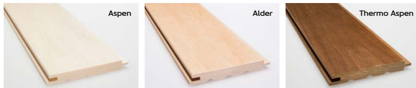
Kallio 15x120 | Thickness: 15 mm | Width: 120 mm | Effective width: 107 mm | Use per square meter 9,4 m | Package size: 6 pcs
