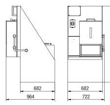
EASYCHLORGEN Standard (Chlorine capacity 280, 560, 1100 or 2200 g/h) All dimensions in mm
