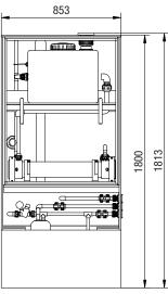
EASYCHLORGEN High Capacity (Chlorine capacity 4250 or 8500 g/h) All dimensions in mm
