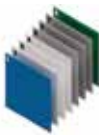
Filter laminate construction according to DIN 18820. Chemical protective barrier made of combination of adequate resin, C-glass veil and glass fibres. Mechanical reinforcement made of combination of spray-up roving, woven roving and radial and helical filament winding. External protective coating in RAL 5015. Other colours upon request with 5% surcharge.
