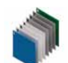
Filter laminate construction according to DIN 18820. Chemical protective barrier made of combination of adequate resin, C-glass veil and glass fibres. Mechanical reinforcement made of combination of spray-up roving, woven roving and radial and helical filament winding.
